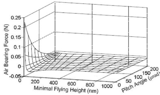
Figure 12: Performance surface of total air bearing force.
