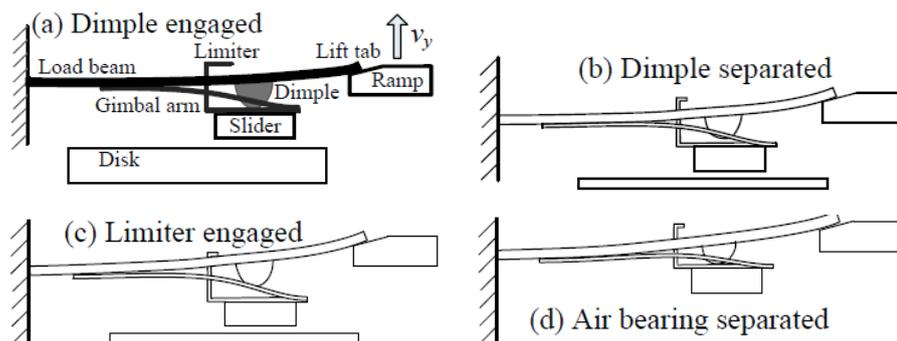
Figure 2: Three stages in unloading processes.
