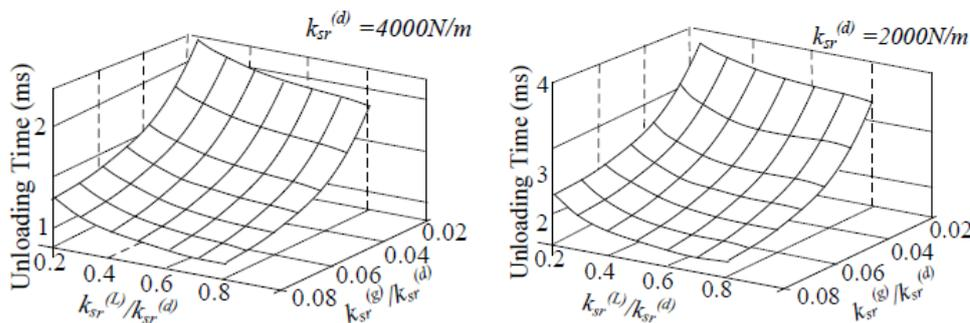
Figure 15: The effects of the stiffnesses on the unloading time.
