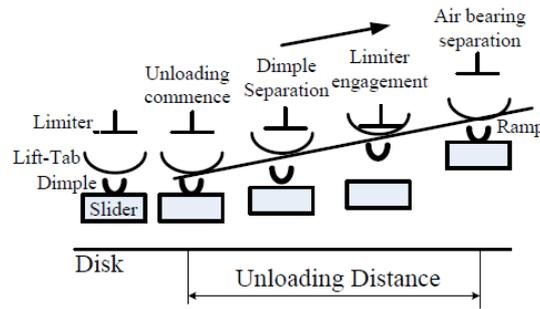
Figure 3: Unloading distance.
