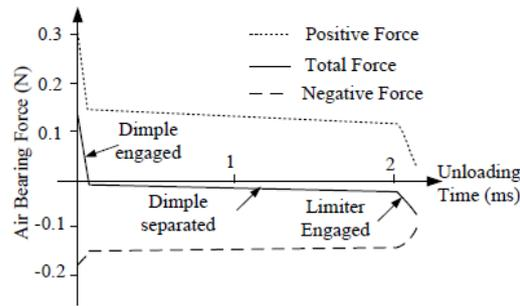
Figure 13: Histories of the air bearing forces in an unloading process.
