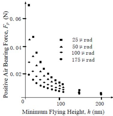
Figure 8:  $F_p$  vs  $h$  for varying pitch angles.
