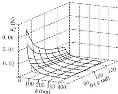
Figure 10: Performance surface of positive air bearing force.
