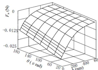
Figure 11: Performance surface of negative air bearing force.
