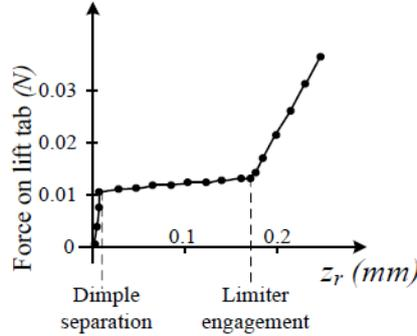
Figure 5: History of the force on the lift tab in the unloading process.
