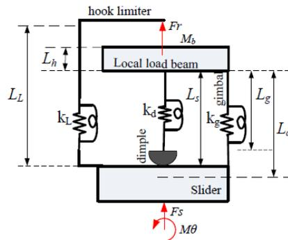
Figure 4: A local lumped parameter suspension model.
