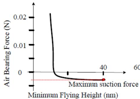
Figure 14:  $F_a$  vs  $h$  in an unloading process.
