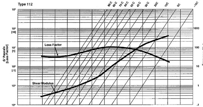
Figure 1: Reduced frequency nomogram for ISD-112.
