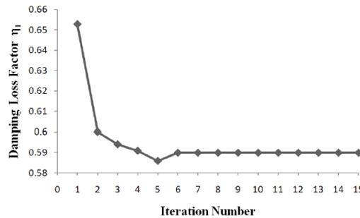
Figure 6: Iteration results for the damping loss factor of mode 1.
