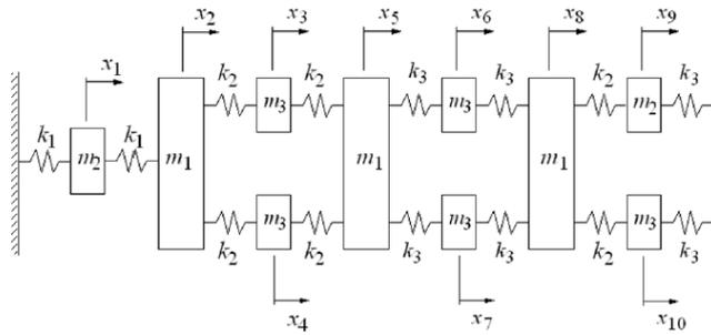
Figure 2: A mass-spring vibration model used as numerical example with  $m_1 = 1.0\text{kg}$ ,  $m_2 = 0.2\text{kg}$ ,  $m_3 = 0.1\text{kg}$ ,  $k_1 = 1.0 \times 10^6\text{N/m}$ ,  $k_2 = 2.0 \times 10^6\text{N/m}$ .
