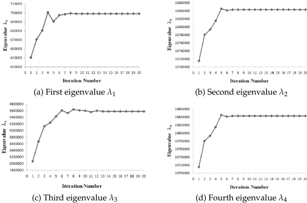
Figure 3: Iteration results showing convergence of the lower 4 modes.
