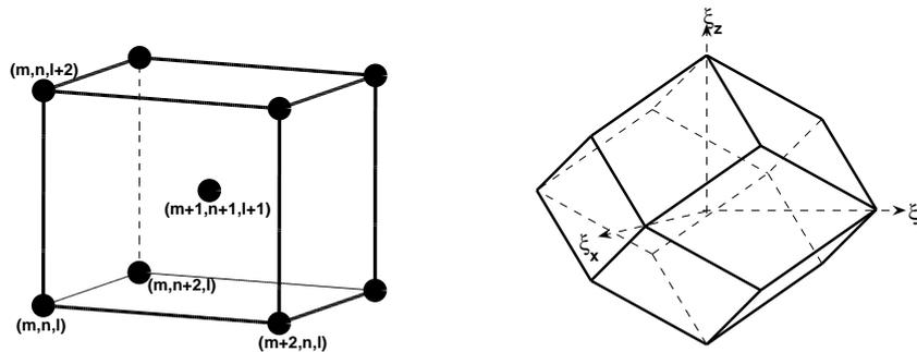
Figure 1: Unit cell (left) and first Brillouin zone (right) of BCC lattice.
