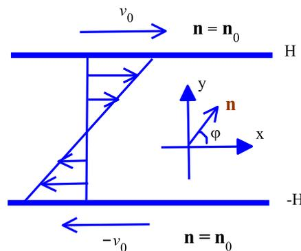
Figure 2: Plane shear flow geometry. The boundary anchoring for the director is assumed to equal to its quiescent nematic equilibrium value and the velocity boundary condition is no-slip  $v(\pm H) = 0$ . The director field  $n$  is measured by the orientation angle  $\varphi$  such that  $\varphi = 0$  is parallel to the walls, and  $\varphi = \pi/2$  is perpendicular.
