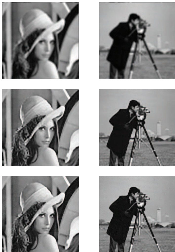
Figure 3: Image restoration results for comparisons between the scheme (4.5) and the split Bregman method with \beta_1 = \beta_2 = 0.04 . (top): Degraded images (convolved with a 9 \times 9 uniform kernel, and then degraded by a zero mean Gaussian noise with derivation \sigma = 0.56^2 ); (middle): Restored images by the scheme (4.5); (middle left): SNR=15.39dB, time=31.37s; (middle right): SNR=15.83dB, time=34.61s; (bottom): Restored images by the scheme (4.11); (bottom left): SNR=15.16dB, time=33.64s; (bottom right): SNR=15.56dB, time=39.08s.
