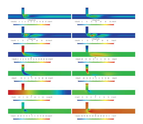
Figure 7: First four basis functions for velocity (first two rows),temperature (rows three and four) and pressure (last two rows) corresponding to  $\theta_m = 60^{\circ}$ C and  $\theta_b = 80^{\circ}$ C.
