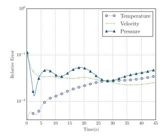
Figure 5:  $\epsilon_{L^2}(t) \operatorname{error} (\epsilon_{L^2}(t) = \frac{||X_{FOM}(t) - X_{ROM}(t)||_{L^2(\Omega)}}{||X_{FOM}(t)||_{L^2(\Omega)}})$  plots for temperature, velocity and pressure fields obtained on the test case for temperature inlet boundary conditions  $\theta_m = 60^{\circ}$ C and  $\theta_b = 80^{\circ}$ C.
