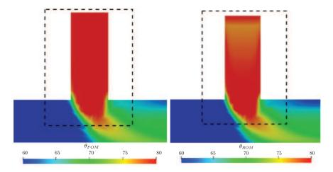
Figure 9: Zoom of the area with the biggest relative error between the FOM (left) and the ROM (right) for temperature field. The temperature inlets are  $\theta_m = 60^{\circ}$ C and  $\theta_b = 80^{\circ}$ C.
