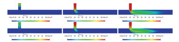
Figure 10: Comparison of the full order field (top row) and temperature reduced order model (bottom row) for the case of temperature inlets  $\theta_m = 20^{\circ}$ C and  $\theta_b = 40^{\circ}$ C. The fields are depicted for different time instances equal to t = 3s,10s and 45s and increasing from left to right.
