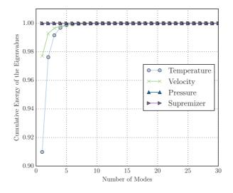
Figure 4: Cumulative energy of the eigenvalues for temperature, velocity, pressure and supremizer fields for the training case with temperature inlet boundary conditions  $\theta_m = 50^{\circ}$ C and  $\theta_b = 70^{\circ}$ C.
