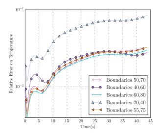
Figure 6:  $\epsilon_{L^2}(t) \operatorname{error} (\epsilon_{L^2}(t) = \frac{||X_{FOM}(t) - X_{ROM}(t)||_{L^2(\Omega)}}{||X_{FOM}(t)||_{L^2(\Omega)}})$  for different temperature inlet conditions. The ROM is trained on  $\theta_m = 50^{\circ}$ C and  $\theta_b = 70^{\circ}$ C and then is used to predict the temperature, velocity and pressure fields on four different test cases with sets of temperature inlets.
