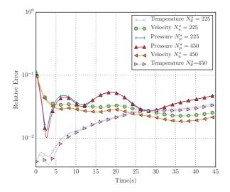
Figure 3:  $\epsilon_{L^2}(t) \operatorname{error} (\epsilon_{L^2}(t) = \frac{||X_{FOM}(t) - X_{ROM}(t)||_{L^2(\Omega)}}{||X_{FOM}(t)||_{L^2(\Omega)}})$  for two sampling frequencies for the snapshot collection, per 0.2s where  $N_u^s = N_\theta^s = N_p^s = 225$  and per 0.1s where  $N_u^s = N_\theta^s = N_p^s = 450$ s. The ROM is run on  $\theta_m = 50^{\circ}$ C and  $\theta_b = 70^{\circ}$ C.
