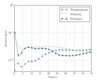
Figure 13:  $\epsilon_{L^2}(t) \operatorname{error} (\epsilon_{L^2}(t) = \frac{||X_{FOM}(t) - X_{ROM}(t)||_{L^2(\Omega)}}{||X_{FOM}(t)||_{L^2(\Omega)}})$  for temperature, velocity and pressure fields for the test case with kinematic viscosity  $\nu = 1.1e - 05$ .
