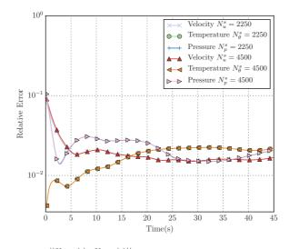
Figure 11:  $\epsilon_{L^2}(t)$  error  $(\epsilon_{L^2}(t) = \frac{||X_{FOM}(t) - X_{ROM}(t)||_{L^2(\Omega)}}{||X_{FOM}(t)||_{L^2(\Omega)}})$  for two sampling spaces for the parameter (kinematic viscosity). These correspond to one with 5 sampling points for viscosity, where  $N_u^s = N_\theta^s = N_p^s = 2250$  and one with 10 sampling points where,  $N_u^s = N_\theta^s = N_p^s = 4500$ s. The ROM is run for  $\nu = 1.1e - 05$ .
