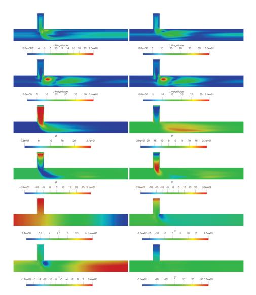
Figure 14: First four basis functions for velocity (first two rows),temperature (rows three and four) and pressure (last two rows) corresponding to  $\nu = 1.1e - 05$ .
