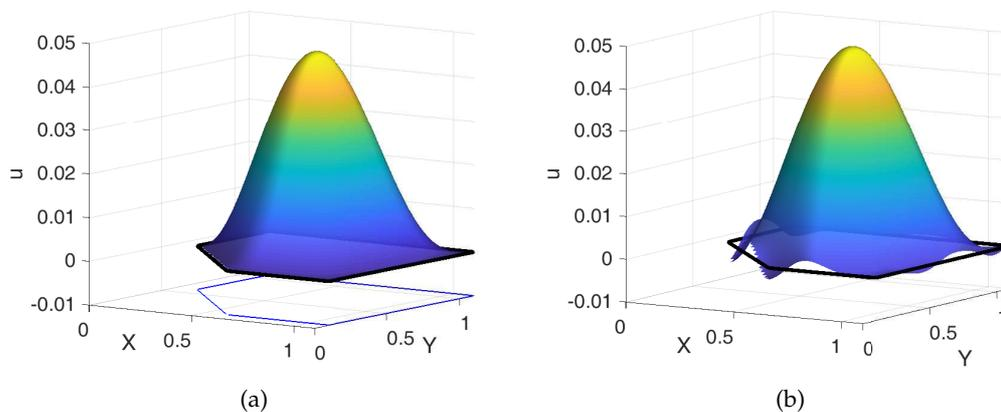
Figure 9: Example 3.4: The profiles of the approximate solution using (a) ghost points and SVD and (b) the traditional Kansa method.
