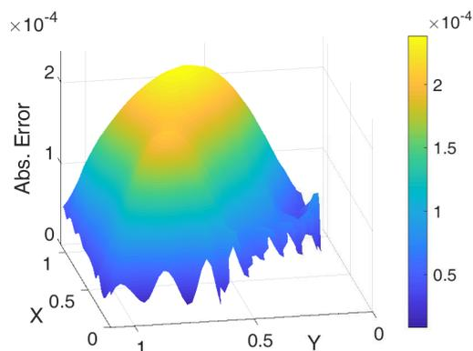
Figure 10: Example 3.4: The profile of the absolute error with respect to the results obtained using COMSOL.
