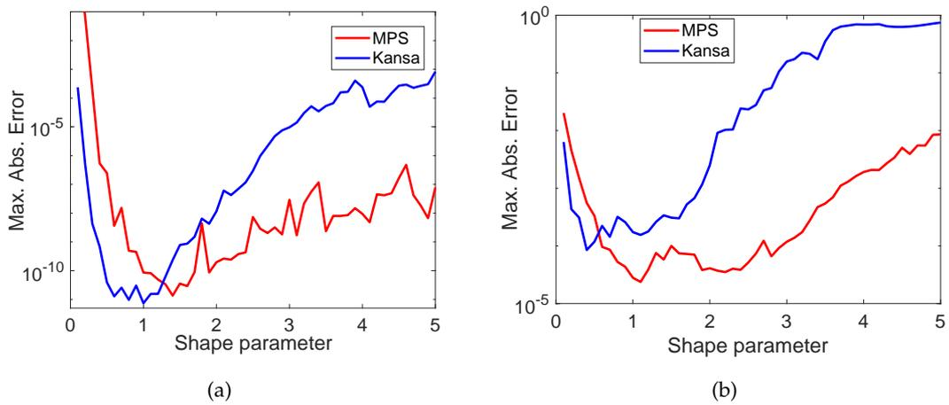
Figure 3: Example 3.1: The maximum absolute errors versus the shape parameter (a) using the ghost points; (b) without the ghost points.
