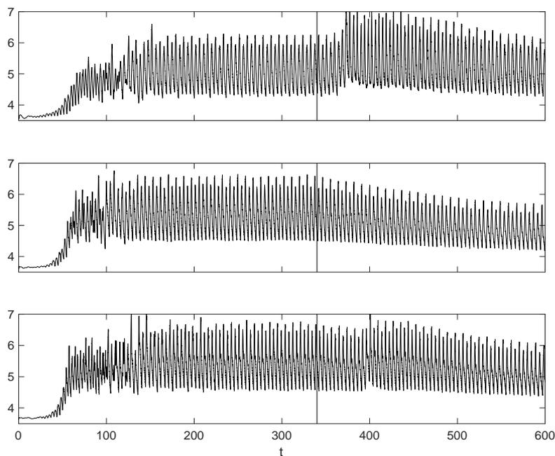
Figure 7: The records of the maximum pressure obtained from simulations on three two-dimensional meshes, which have 25600, 102400, 409600 cells. The vertical line at  $t \approx 340$  denotes the reliable period.
