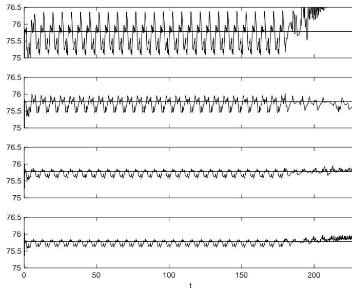
Figure 3: Maximum pressure curves obtained from simulations with the configuration given by Example 4.1. The numbers of grid points in  $L^{1/2}$  are, from top to bottom, 20, 40, 80, 160 with  $L = 300$ , respectively. The reliable period is 182 in this case
