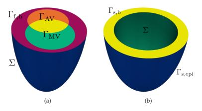
Figure 3: Fluid (a) and structure (b) meshes for the prolate ellipsoid (tests A, B and C)
