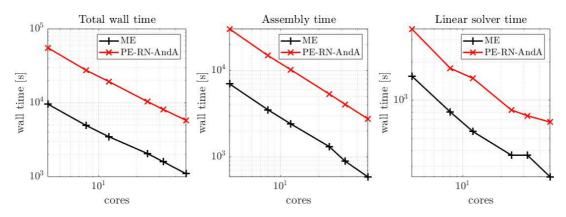
Figure 7: Comparison of ME and PE-RN-AndA schemes with varying number of cores. From left to right, we report the total wall time, the time spent for assembly and the time spent for solving linear systems. Refer to Table 2 for an explanation of the abbreviations used.
