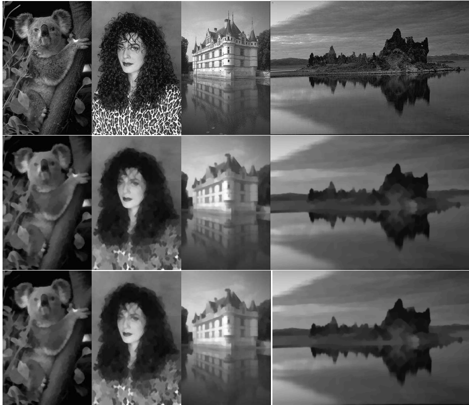
Figure 3: Four input images are shown in the first row; the computed images u^*(x) are given in the 2nd row, respectively; the rounded images u^*(x) are shown in the 3rd row, respectively. In all experiments, we set \alpha = 0.5 .
