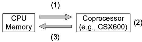
Figure 2: How to use a coprocessor. (1) Transfer data from memory to a coprocessor (2) Compute matrix-matrix multiplications (3) Transfer computational results to memory.
