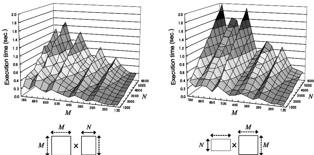
Figure 5: The execution time of matrix-matrix multiplications on the CSX600 coprocessor. The left figure shows the time for multiplying a  $M \times N$  real matrix by a  $M \times M$  real matrix from left. The right figure shows the time for multiplying a  $N \times M$  real matrix by a  $M \times M$  real matrix from right. The execution time roughly changes especially with respect to  $M$  even though the computational work is proportional to  $M^2N$  in both cases.
