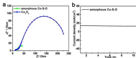
**Figure 4.** (a) Nyquist plots of different electrodes at an overpotential of 300 mV for HER; (b) Chronoamperometric response of amorphous Co-S-O in 1 M KOH solution at the applied potential of 1.52 V versus RHE.
