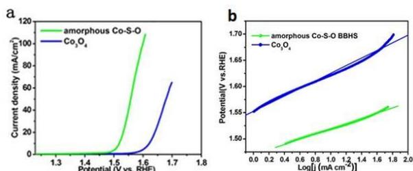
**Figure 3.** (a) polarization curves for OER at a scan rate of 10 mV s<sup>-1</sup> in 1.0 M KOH and (b) corresponding Tafel plots.
