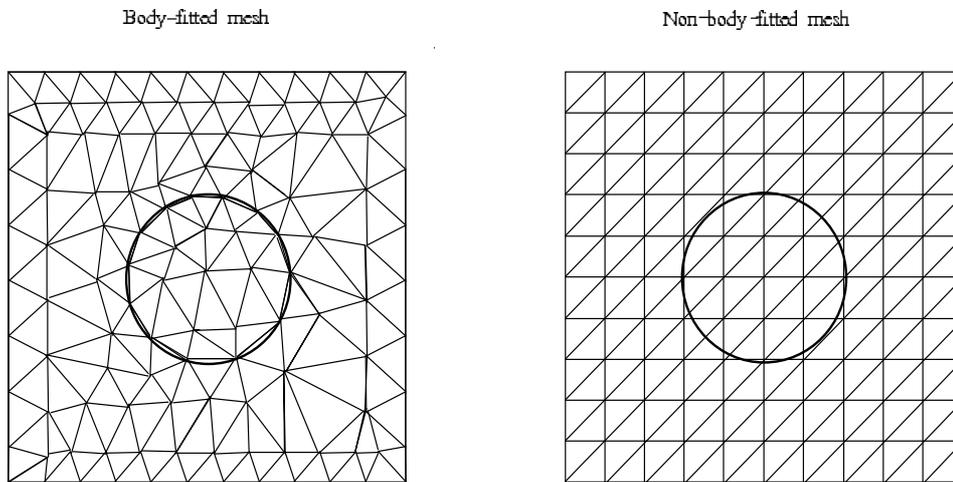
Fig. 1.1. The body-fitted and non-body-fitted mesh in 2D.
