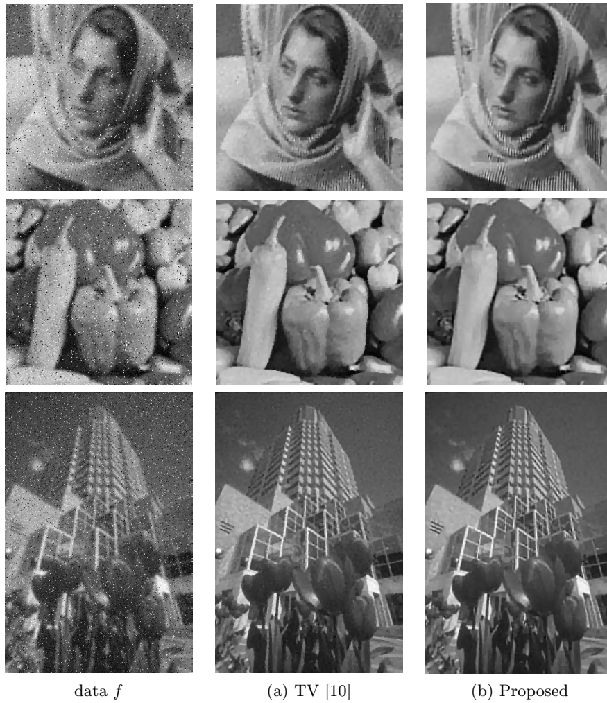
Fig. 4.2. Deblurred and denoised images when data f degraded by a uniform blur and Cauchy noise with \gamma = 5 . (a) TV model [10], (b) Our model. PSNR (top to bottom row): (a) 24.485/28.159/25.037, (b) 25.403/28.858/25.575. Parameter \lambda for our model: (top to bottom) 1950, 1800, 1900.
