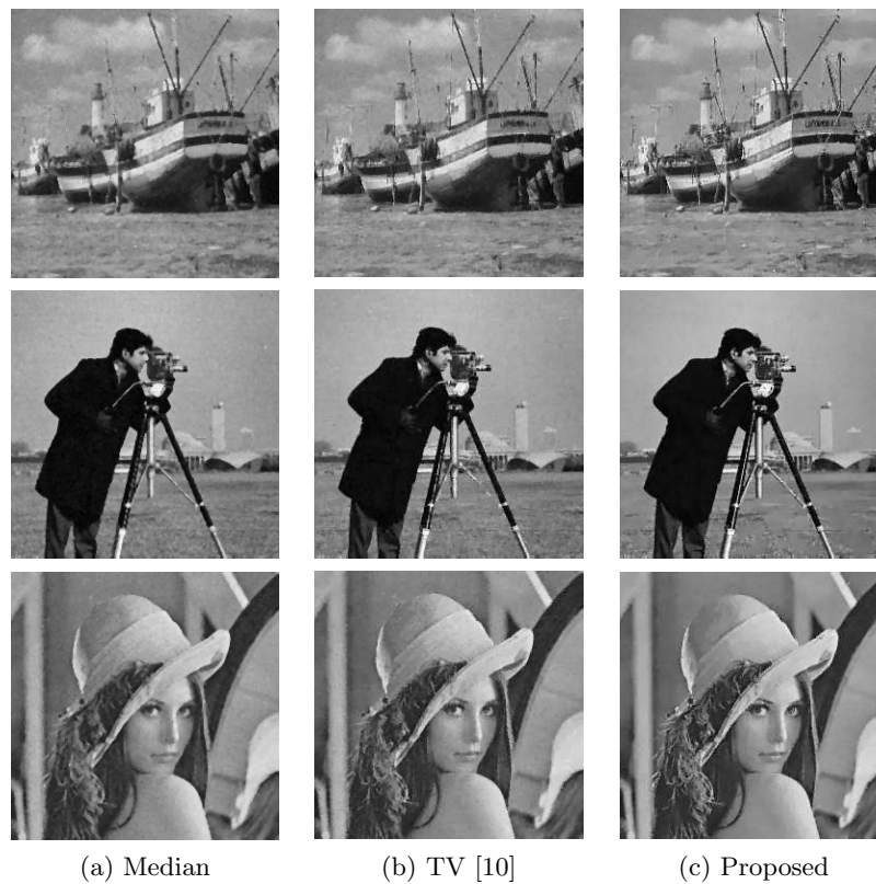
Fig. 3.10. Denoised images when noise level \gamma = 5 , using (a) Median filtering, (b) TV model [10], (c) our model (3.2). PSNR (from (a) to (c)): (top) 25.168/26.894/28.730, (middle) 26.272/27.721/30.026, (bottom) 28.387/29.434/31.043. Parameter \lambda for our model: (top to bottom) 600, 550, 550.
