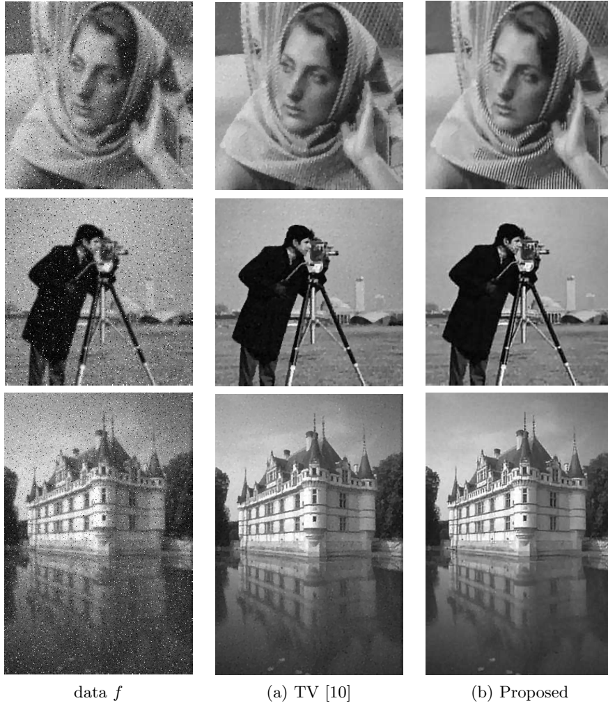
Fig. 4.1. Deblurred and denoised images when data f degraded by a Gaussian blur and Cauchy noise with \gamma = 5 . (a) TV model [10], (b) Our model. PSNR (top to bottom row): (a) 24.924/26.662/27.075, (b) 27.239/27.511/27.903. Parameter \lambda for our model: (top to bottom) 1500, 1400, 1350.
