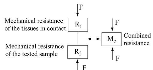
Figure 2 Equivalent mechanical sensing system
