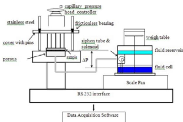
Figure 1 Gravimetric Absorbency Testing System (GATS)
