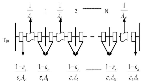
Figure 2 Radiative heat transfer diagram
