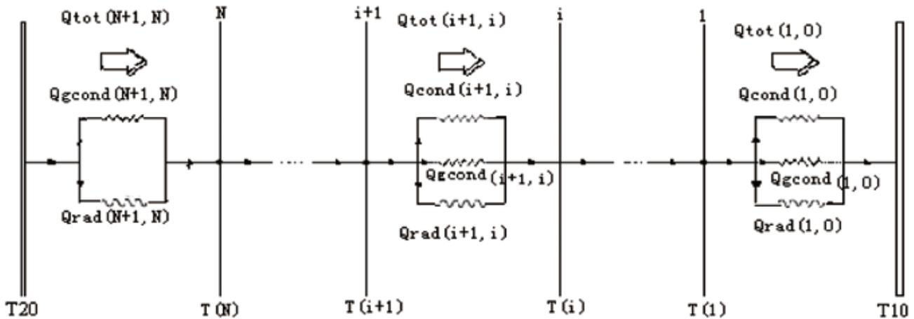
Figure1 Model structure, input and output parameters of thermal network
