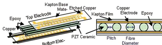
Figure 1 Piezoelectric fibre composite.
