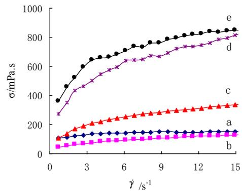
Figure1 The effect of shear rates on shear stress of urea denatured soybean protein. a-0 mol L<sup>-1</sup> Urea, b- 2 mol L<sup>-1</sup> Urea, c- 4 mol L<sup>-1</sup> Urea, d- 6 mol L<sup>-1</sup> Urea, e-10 mol L<sup>-1</sup> Urea(20 °C SPI 10 wt%).
