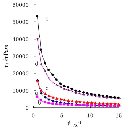
Figure 2 The effect of shear rates on apparent viscosity of urea denatured soybean protein. a-0 mol L<sup>-1</sup> Urea, b- 2 mol L<sup>-1</sup> Urea, c- 4 mol L<sup>-1</sup> Urea, d- 6 mol L<sup>-1</sup> Urea, e-10 mol L<sup>-1</sup> Urea(20 °C SPI 10 wt%).
