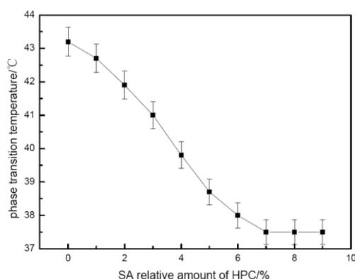
Figure 1 Effect of SA amount on phase transition temperature of HPC/SA blends.
