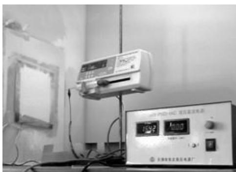
Figure 1 System setup for electrospinning process.
