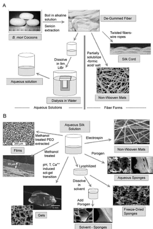
Figure 1. (A) Silk fibroin is purified from sericins via boiling in an alkaline solution. (B) Processing of silk morphologies from aqueous silk fibroin solution [17].
