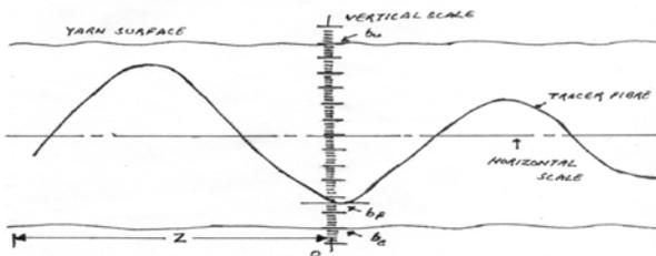
Figure 2 Migration Behavior of Tracer Fibre in the yarn.
