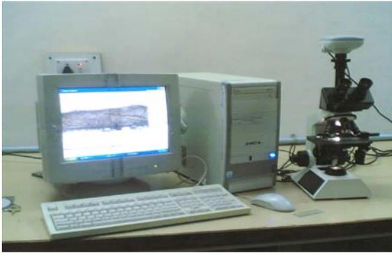
Figure 1 Computerized high power binocular microscope with CCD camera attachment.
