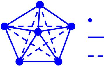
Figure 1 Mass-spring system with Tension-Shear springs (solid lines), and bending springs (dash lines).
