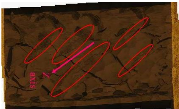
(c) Morphology of connecting yarns with resin cover
