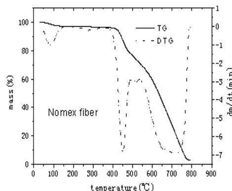
Figure 2 The TG and DTG curves of Nomex fiber.
