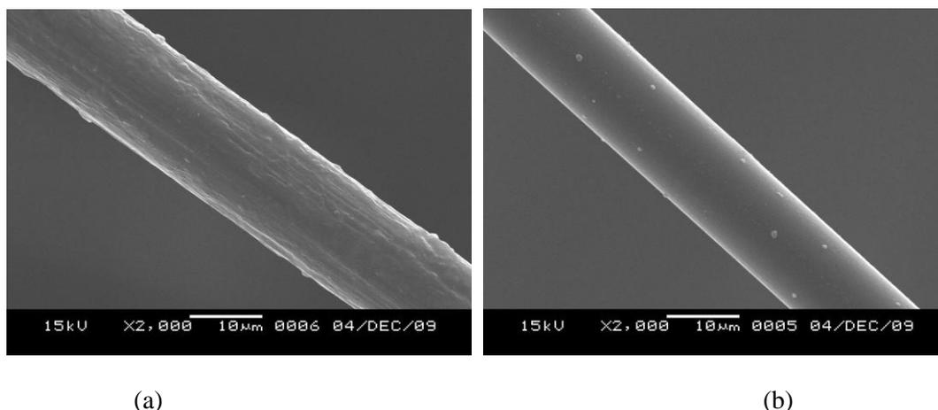
Figure 1 Longitudinal micrographs of Nomex and Kevlar 49 fiber. a Nomex fiber. b Kevlar 49 fiber.
