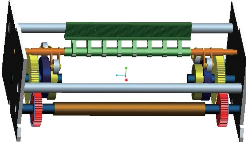
Fig. 1: Parameterized model of beating-up mechanism
