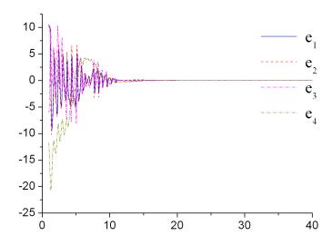
Fig.1.Synchronization errors of the delay hyperchaotic Lüsystem.
