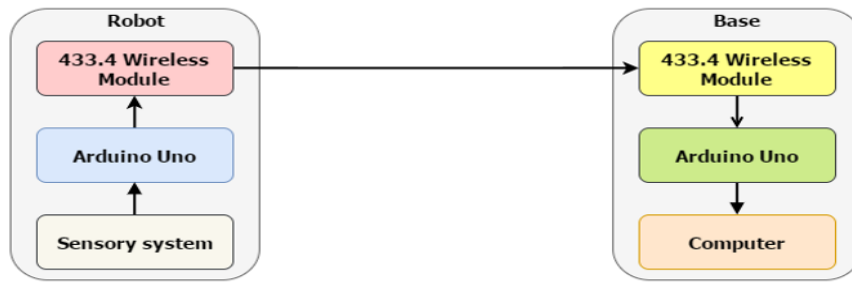
Fig.17. Block diagram of the communication channel between the two Arduino Uno.
