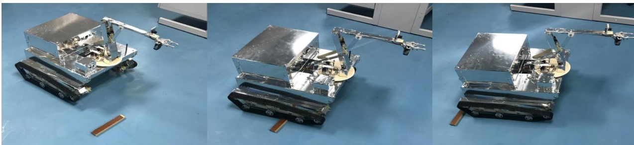
Fig.35. Climbing small obstacles test.
