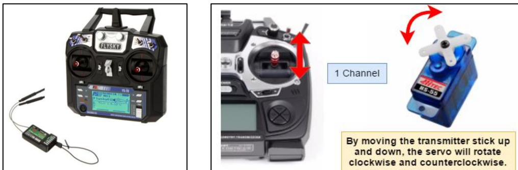
Fig.14. (a) FLYSKY FS-i6 (transmitter/receiver) (b) The control of a single channel
