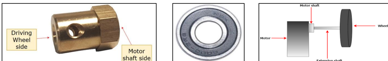
Figure 4: (a) Coupling shaft. (b) The used bearings (c) Motion system
