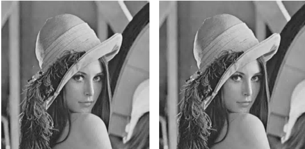
(c) Decoded with Quality=0.06, PSNR=33.1 dB (d) Decoded with Quality=0.08, PSNR=31.7 dB
