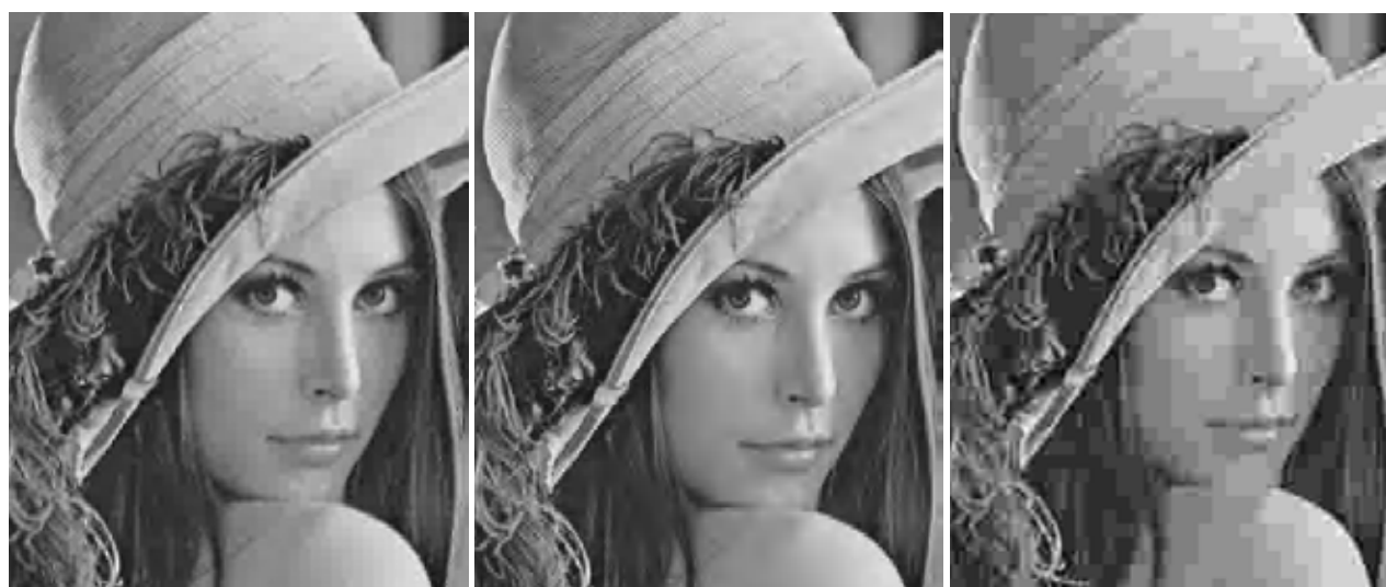
(j) Decoded by Our Approach Quality=0.08, PSNR=31.7 dB
