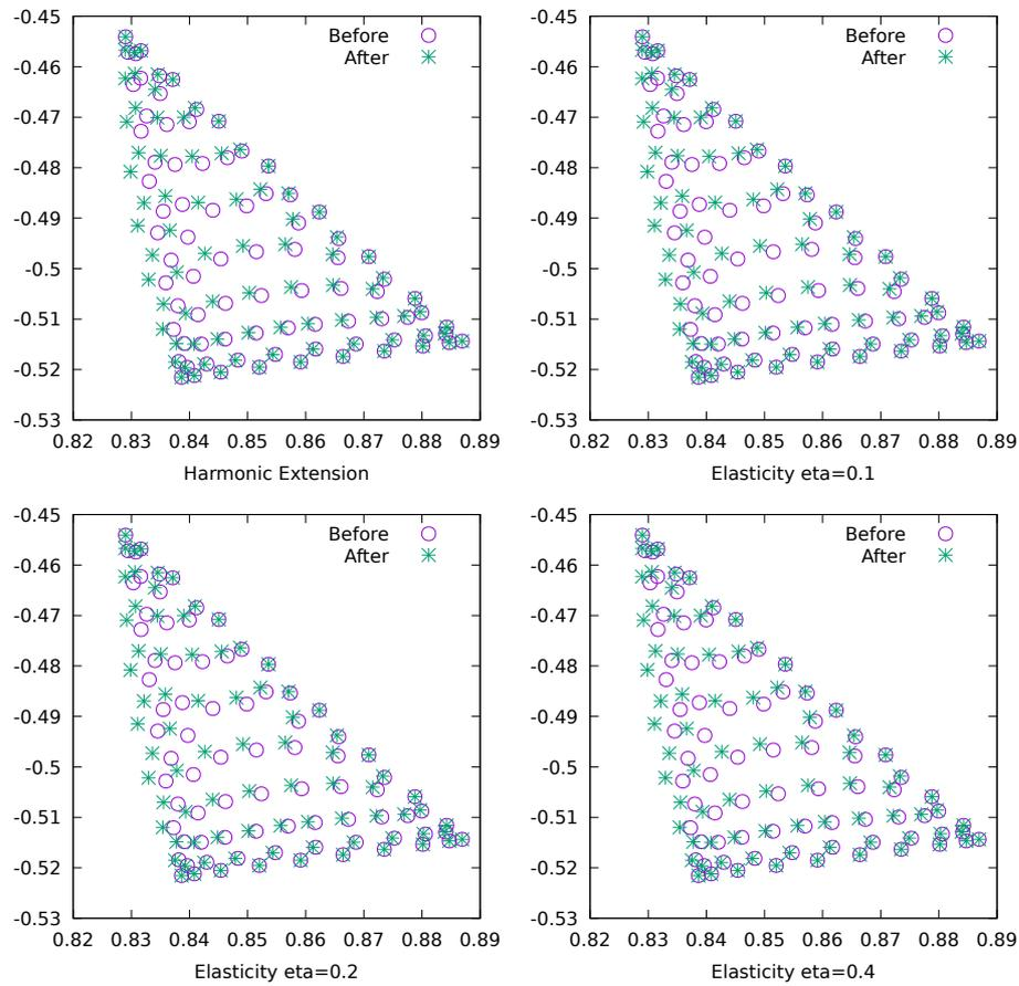
Figure 4: Distribution of the cubature nodes before and after the isoparametric mapping: Harmonic extension (top left), elasticity with  $\eta=0.1$  (top right),  $\eta=0.2$  (bottom left) and  $\eta=0.4$  (bottom right).
