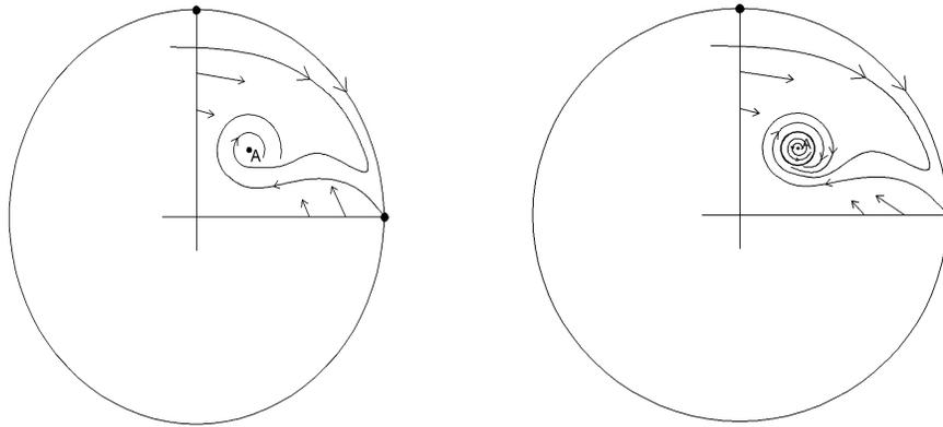
(a) The trajectories approach a singular point. (b) The trajectories approach a limit cycle.
