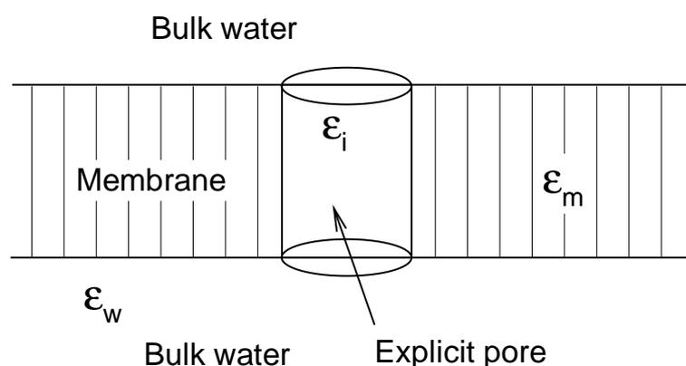
Figure 1: Schematic illustration of an ion-channel model. The molecules inside the cylindrical pore are treated explicitly at the atomic scale, while outside the pore the membrane and water are treated as homogeneous media, characterized by dielectric constants  $\epsilon_m$  and  $\epsilon_w$ , respectively.
