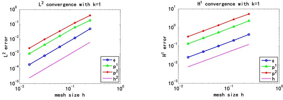
Fig. 5.5. h-convergence on mixed-polygon mesh with  $t = 1.0$ .
