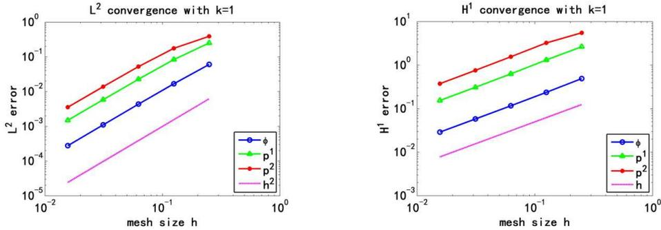
Fig. 5.4. h-convergence on non-convex mesh with  $t = 1.0$ .
